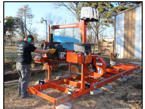
Dan cutting a log into slab on Wood Mizer Sawmill
