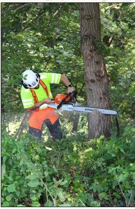
Philip Kelley demonstrating a proper notching technique when felling a tree.
