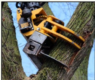
Grapple saw cutting a large tree branch at same time it holds onto the branch.
