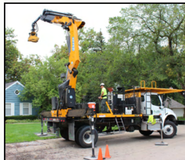
Grapple saw and the EFFER crane truck configuration.
