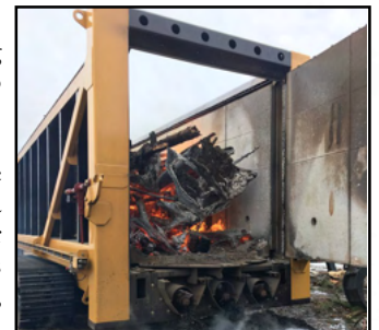
Biomass is burned to produce Biochar
